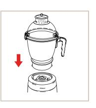
After fitting suitable blade, fill the jar with the ingredients to be processed (don't fill it more than the recommended quantity). Cover the jar with Lid / dome. Carefully insert the jar on to the Motor Unit. Ensure that Locks of the jar slide down the slots of the Motor Unit.
