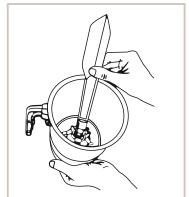
To fit the dry grinding blade on the shaft in the jar, hold the Nylon coupler on the underside of the jar with one hand, and with the help of the spanner (provided in the handle of the spatula) tighten by rotating it anti clockwise till the blade is securely fastened.
