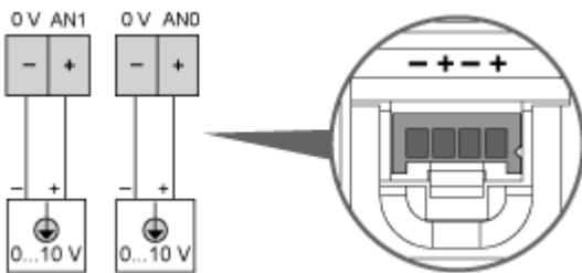
The (-) poles are connected internally.
